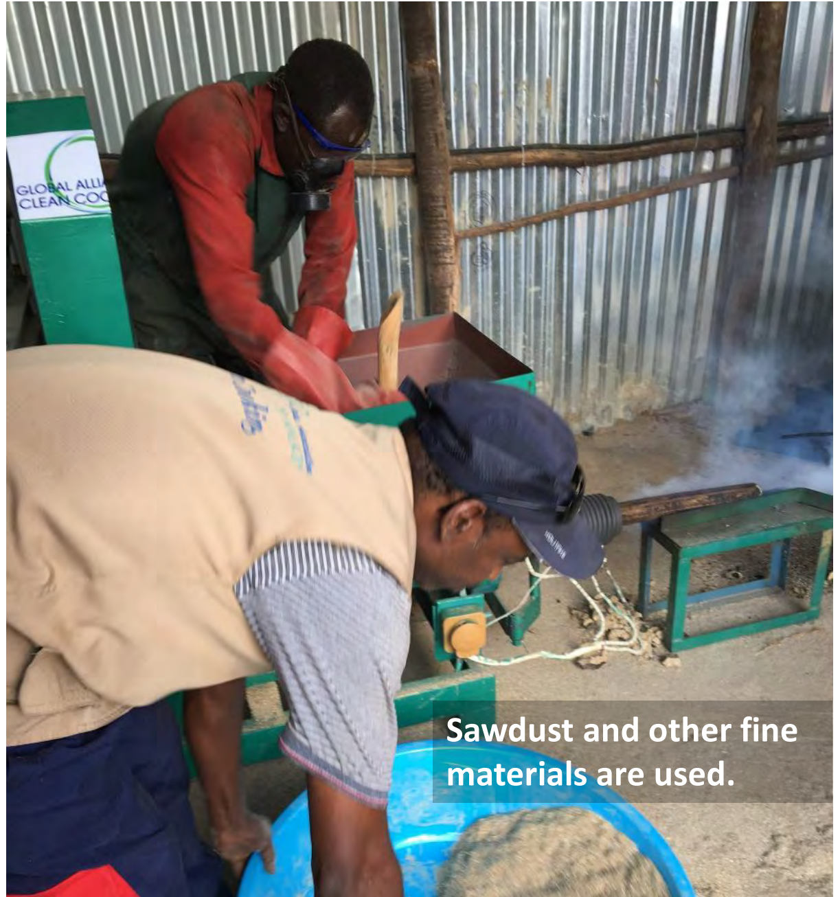
The extrusion process produces heat and fuses the sawdust into logs.
